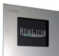
The Home-Icon TouchScreen from Futronix features a TFT (Thin Film Transistor) touch screen with interactive graphics.
