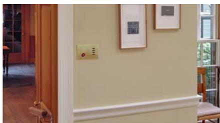
Control switchplates are the typical method of controlling Futronix intelligent lighting systems. Commonly wall-mounted near a room entrance, a switchplate provides a convenient way to program and cue lighting scenes.
